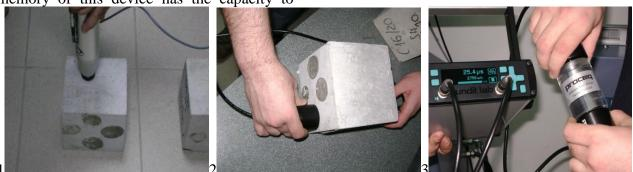
Figure 6. Images from the tests: 1. Digi Schmidt, 2. Pundit Lab, 3. Pundit Lab device calibration
