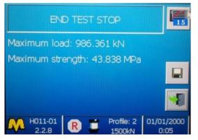
Figure 9. Results displayed on the main unit of universal press
